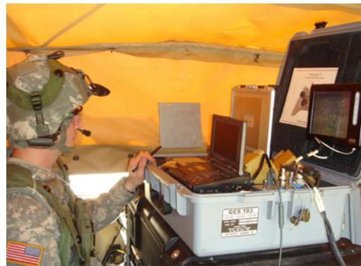
Lockheed Martin's Desert Hawk III small unmanned aircraft system provides the warfighter with an easy-to-use persistent surveillance platform. A portable ground control station with touchscreen laptop allows remote operators to view video transmitted from the air vehicle.
