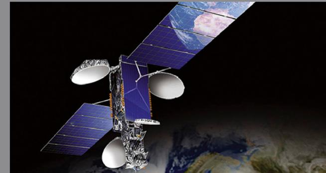
Thruster systems allow A2100s to maneuver into a geosynchronous position, making it possible and cost-effective to launch them in pairs.
