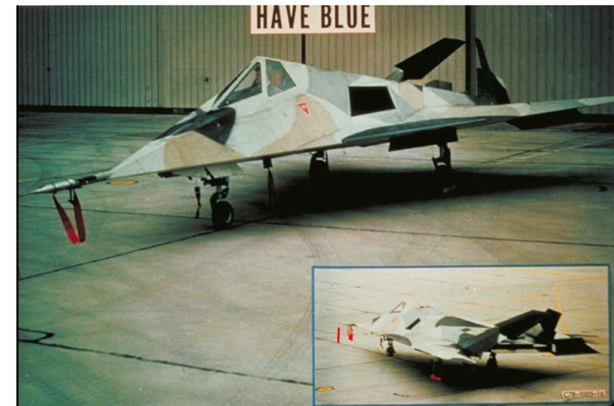
The Have Blue program confirmed that radar signatures low enough to negate battlefield air defense threats could be achieved in a practical flight vehicle. Two aircraft were developed in the mid-1970s, complemented by the development of the first practical computer program, Echo 1, which accurately predicted the radar signature of an air vehicle. The Have Blue program led to the development of the successful F-117A.
