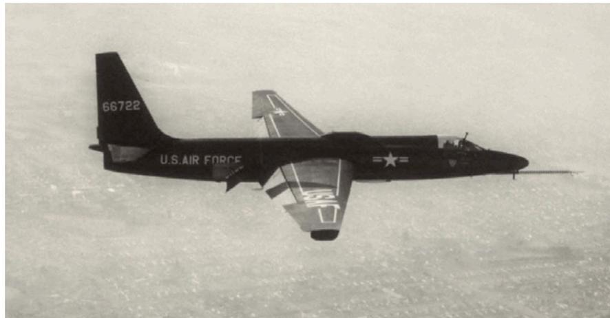
The long, tapered wing of the U-2, shown here in 1955, allowed it to fly 3,000-mile missions and carry up to 700 pounds of photoreconnaissance equipment to a staggering and unprecedented altitude of 70,000 feet.
