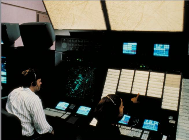
Lockheed Martin's Display System Replacement interfaces with a host computer system to replace end-of-life display generation equipment and gives air traffic controllers modern replacements for aging plan view displays, computer readout displays, and flight data input/output devices, 1995.
