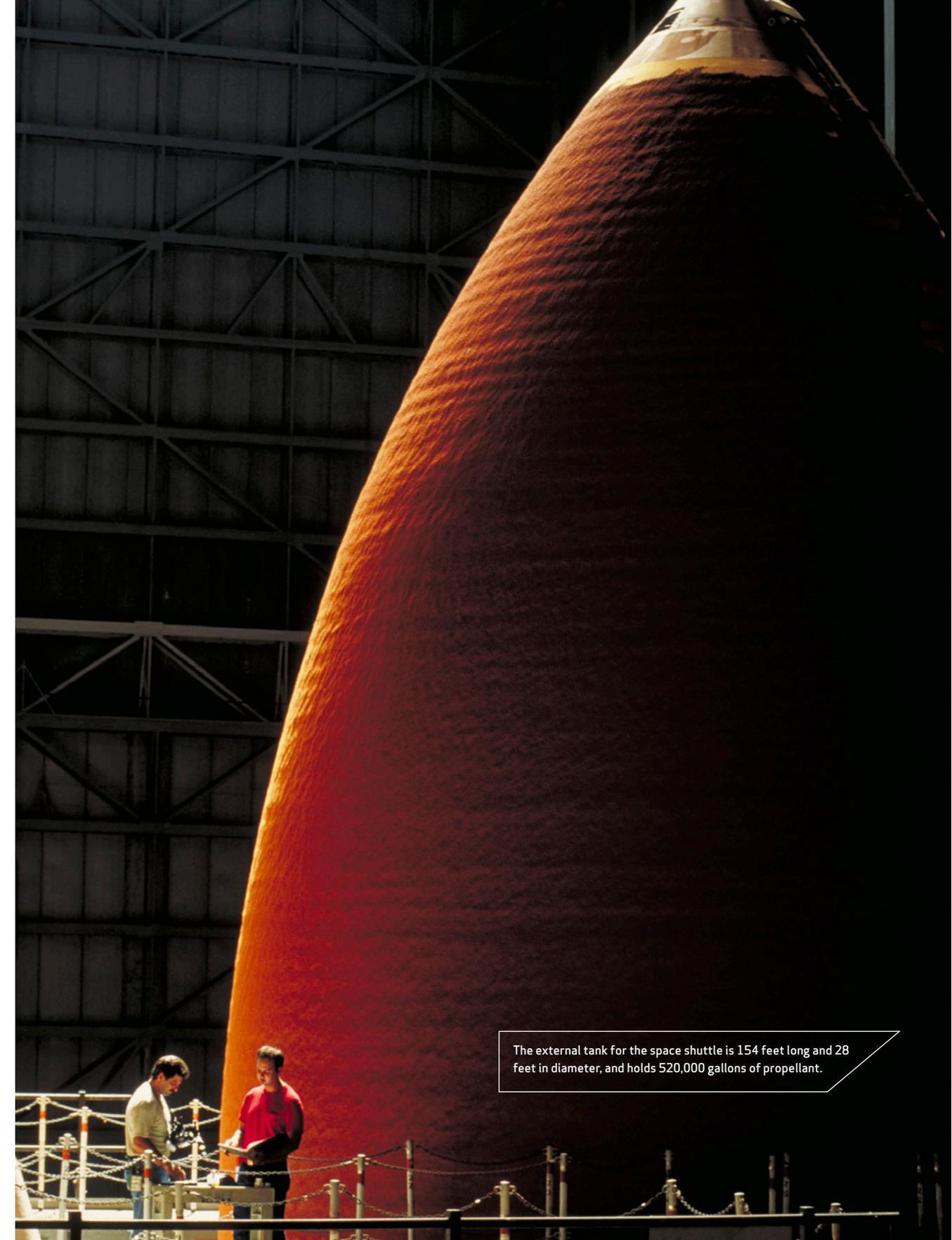
The external tank for the space shuttle is 154 feet long and 28 feet in diameter, and holds 520,000 gallons of propellant.
