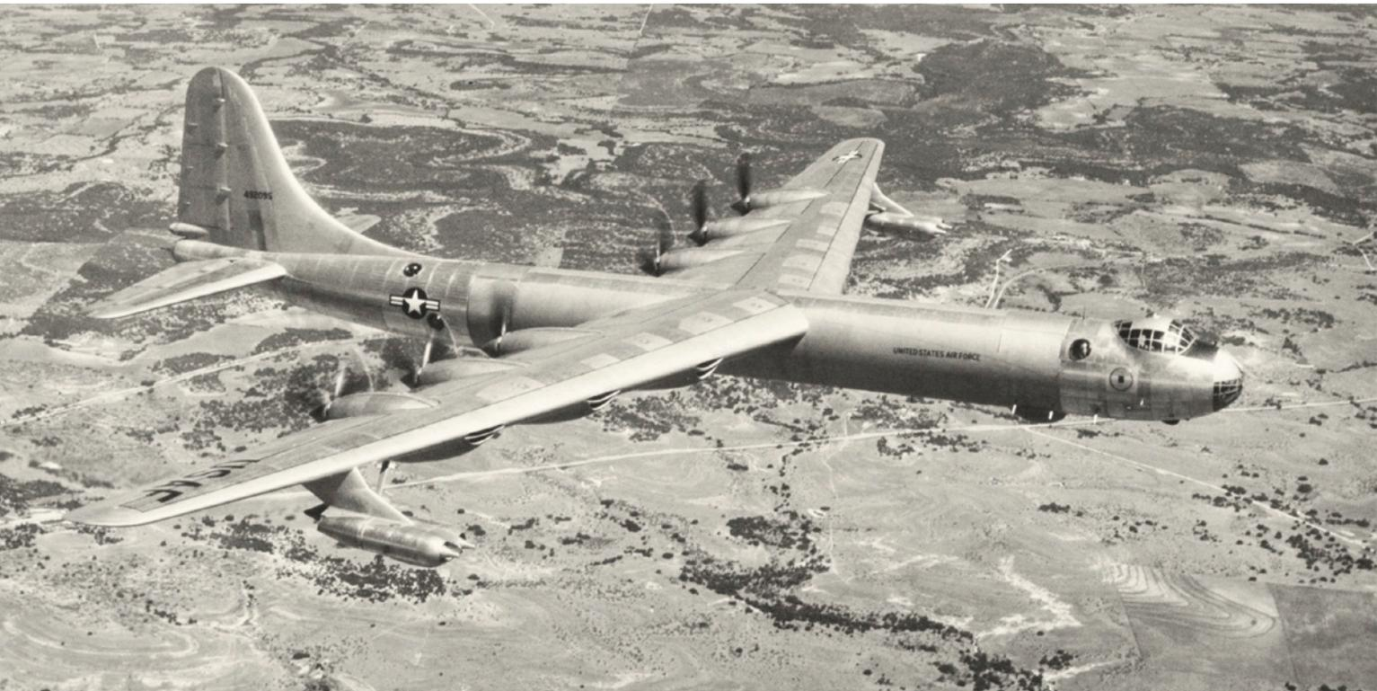
The largest American warplane ever created, the Convair B-36, could fly 4,000 miles with an 80,000-pound payload. The first B-36 was introduced in August 1946. Just three years later, some B-36 models could reach top speeds of 435 mph, a 50,000-foot ceiling, and a range of up to 12,000 miles, solidifying their position as an intimidating long-distance bomber and vital reconnaissance aircraft.
