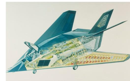
Denys Overholser and Dick Sherrer's computer program had revealed that a diamond-shaped aircraft — what looked on paper like a flying engagement ring — would be 1,000 times less visible to radar than any other aircraft ever created at Lockheed. The flat surfaces, sharp edges and tilted facets of the F-117A's design reflected radar signals away at odd angles, while specially created surface materials absorbed radar energy.
