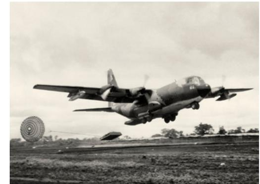
C-130s were perfectly equipped to carry out low-altitude parachute extraction drops of cargo, which led to the plane's key role in the defense of Khe Sanh in 1968. C-130s accounted for 90 percent of the supplies used by troops defending the village against the North Vietnamese siege.
