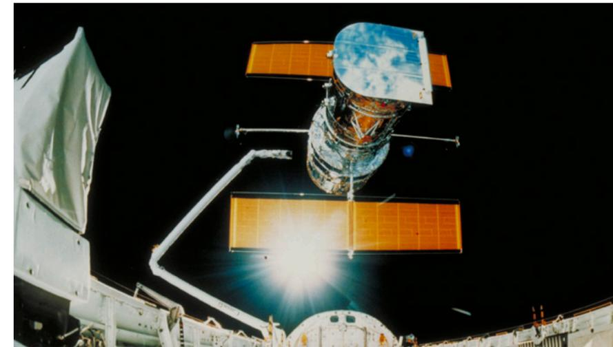
The Hubble Space Telescope was deployed into a 380-mile orbit by the STS-31 crew of the space shuttle Discovery. Photographed just after being released from the Remote Manipulator System robot arm, April 25, 1990.
