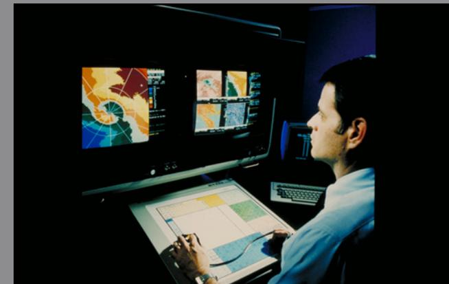
The NEXRAD advanced Doppler weather radar displays radar data on the Principal User Processor. The PUP allows operators to access more than 70 weather products quickly and easily by using the graphic selection tablet, mouse or keyboard. About 160 of the radars are being installed throughout the USA and at selected international locations for the National Weather Service, the Department of Transportation (FAA) and the Department of Defense.
