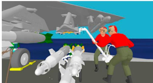
The Human Immersive Lab helped ensure that the design for the underwing fuel drain on the F-35 gave technicians access even when the aircraft is parked tail-over-water on an aircraft carrier. "A one-hour work session can save a retrofit that might cost millions of dollars if caught too late," said Ray Harbor, carrier integration lead for the F-35's Basing and Ship Suitability project.<sup>4</sup>
