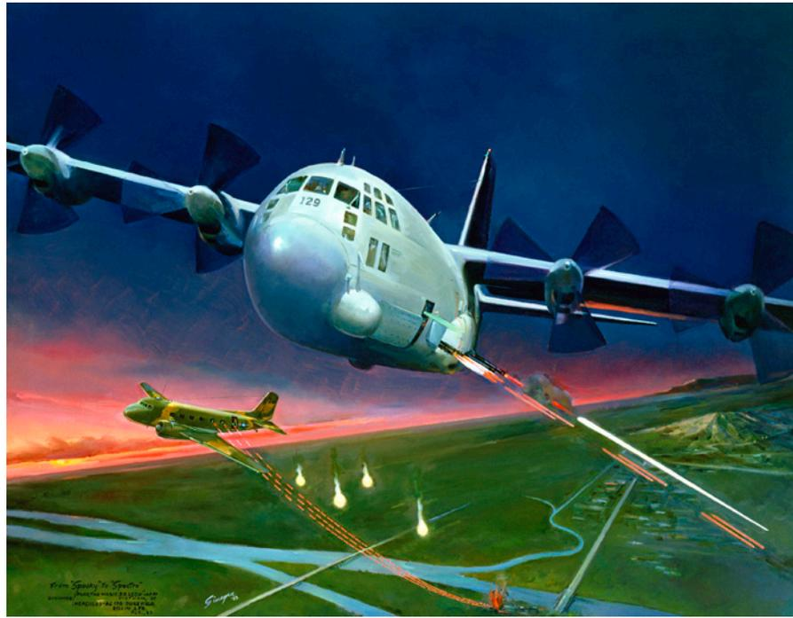
Equipped with ground-target radar, 20 mm Gatling guns, 40 mm cannons, and later, a side-firing 105 mm Howitzer, C-130s morphed into AC-130 gunships, destroying 10,000 enemy trucks and repelling countless enemy attacks in Vietnam. Late in the war, Hercules planes were even being fitted with the largest bomb in the U.S. arsenal, the 15,000-pound BLU-82.
