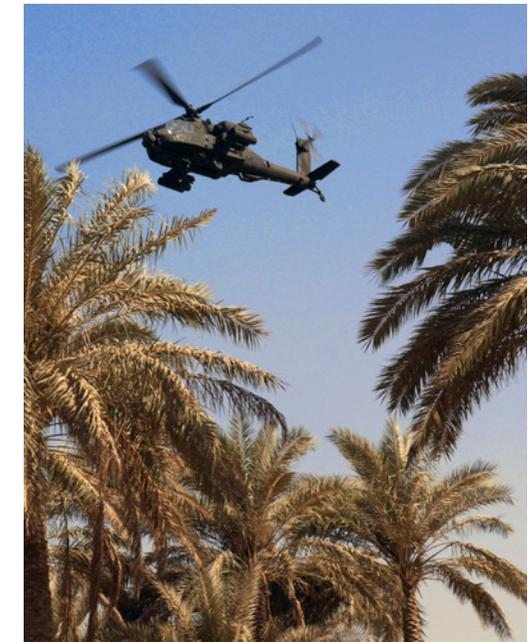
In the early months of the campaign, AH-64 Apache helicopters again took their place as frontline fighters, equipped with a new generation of night vision sensors and thermobaric Hellfire missiles "capable of reaching around corners, striking enemy forces that hide in caves or bunkers and hardened multiroom complexes."<sup>4</sup>
