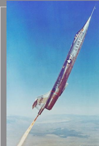
An R-2 rocket fitted above the jet engine boosts the NF-104 Starfighter into the upper atmosphere for high-altitude astronaut training at Edwards Air Force Base, 1957.
