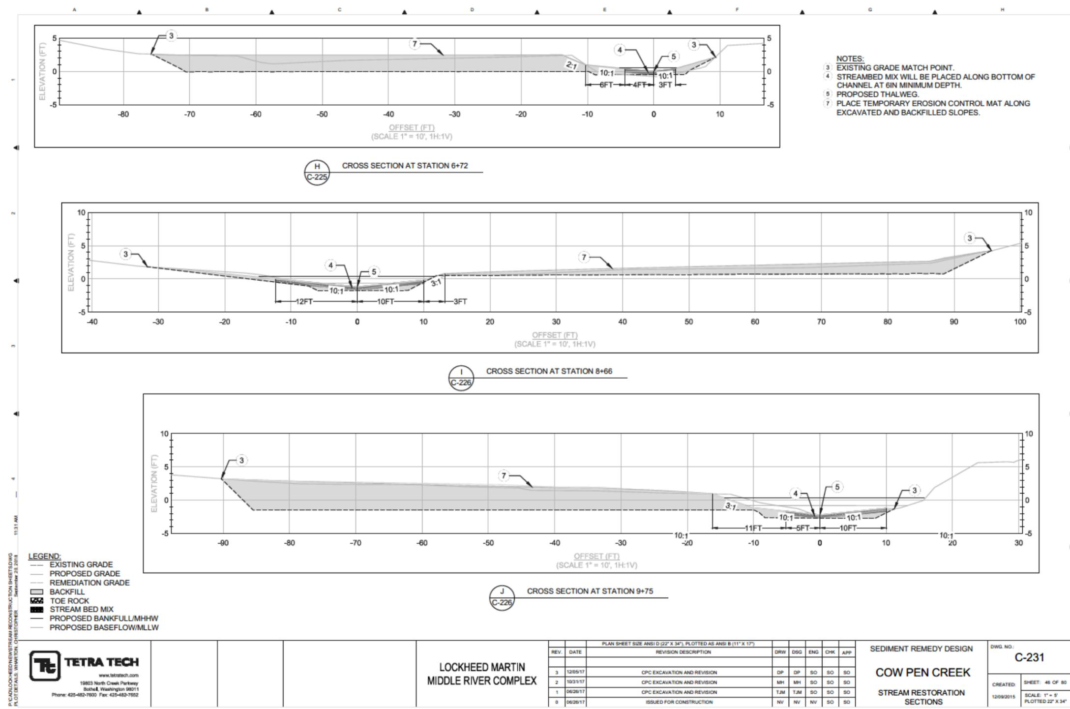
Figure 2-2. Stream and Floodplain Cross-Sections, Cow Pen Creek Restoration
