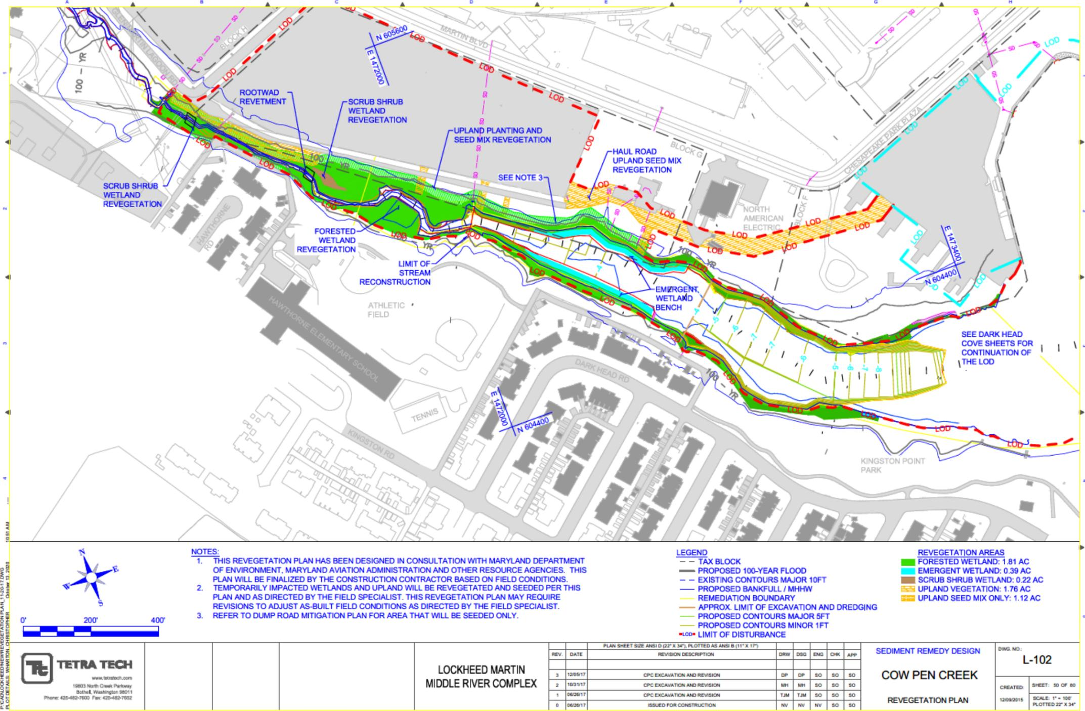
Figure 2-1. Extent of Cow Pen Creek Stream Channel and Floodplain Reconstruction (Source: November 2017 revegetation plan [Tetra Tech, 2017])
