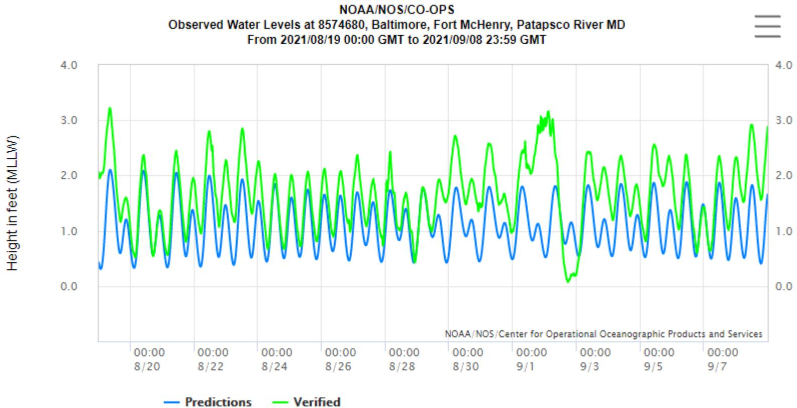
**Figure 3-2. Observed water levels at NOAA’s tidal observation station at Baltimore, Fort McHenry, Patapsco River, August 19 – September 8, 2021.**
