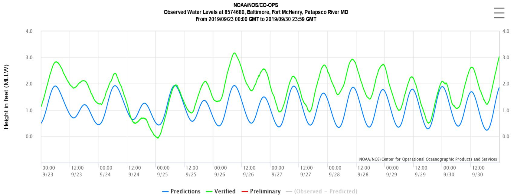
**Figure C – 4. Observed water levels at NOAA tidal observation station at Baltimore, Fort McHenry, Patapsco River September 23-30, 2019**
