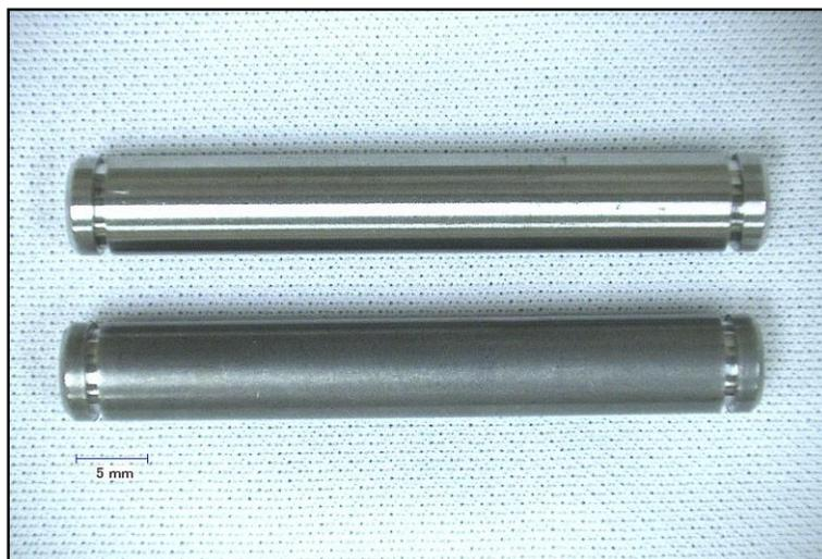
*Figure 6 The bottom pin has aluminum oxide residue.*
