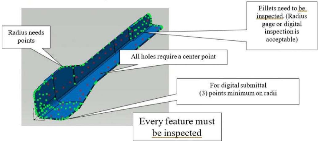
Figure 3 Sample of Validation Points Including Hole Diameters
