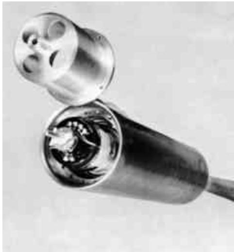
Figure 6-6 Typical Model and Roll Mechanism Assembly
