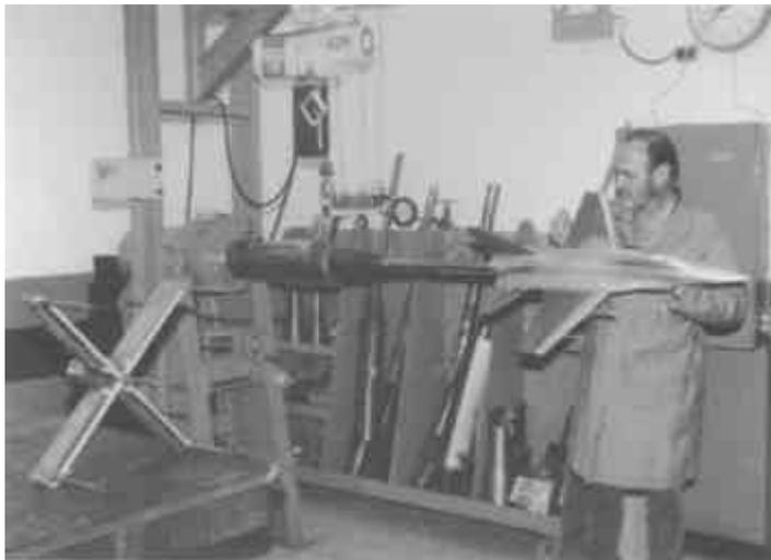
The model setup room, shown in Figure 2-3, is located west of the office areas and contains machine and hand tools for minor model repairs and parts fabrication. Models and related instrumentation are assembled and checked thoroughly in this room prior to installation in the tunnel test section. The model room also offers machine tools for model repair and modification as shown in Figure 2-4.
