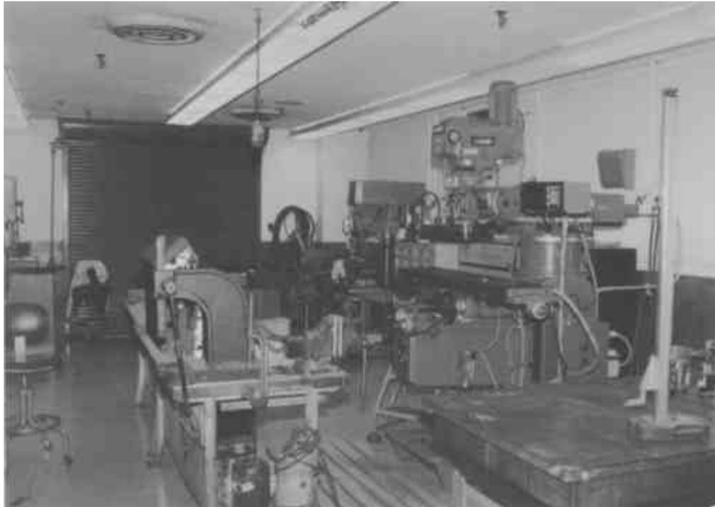
**Figure 2-4 Model Setup Room Machine Shop Tools for Model Repairs and Modifications**
