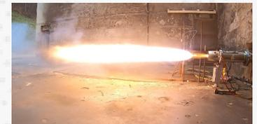
In November 2021, Lockheed Martin successfully completed the first ambient static fire testing for the JAGM-MR solid rocket motor.
