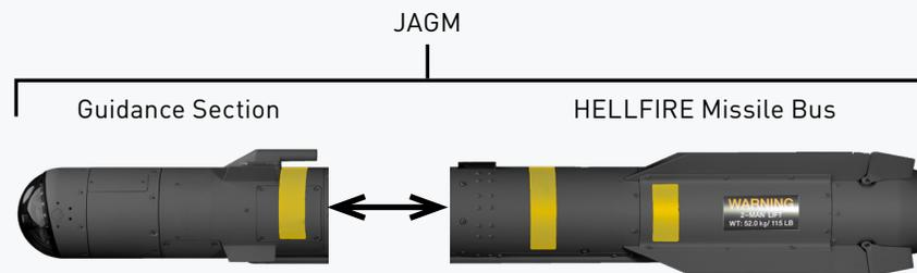
The missile's sensors are integrated into the JAGM guidance section, which is then mated with the AGM-114R multi-purpose HELLFIRE II missile body (including the control actuation system, warhead and rocket motor), capitalizing on missile program improvements that have migrated into the modern HELLFIRE II design.
