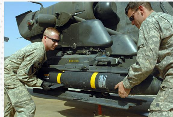
M299 Launcher being loaded with HELLFIRE® Missiles.
