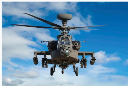
The M299 launcher is deployed on the AH-64D, AH-64E, Seahawk, Cobra, Tigre and numerous other platforms for US and international customers.
