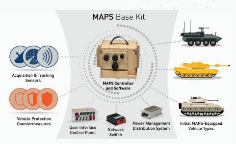
The MAPS open standards-based framework allows users to interchange APS sensors and countermeasures without proprietary interface restrictions.
