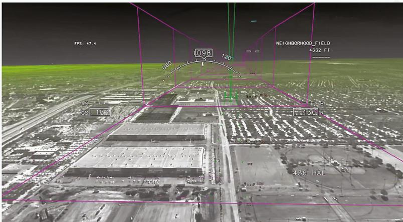
Flight imagery from PDAS' first tactical installation fuses aircraft and DTED data with 360-degree sensor imagery to provide situational awareness and tactical information.
