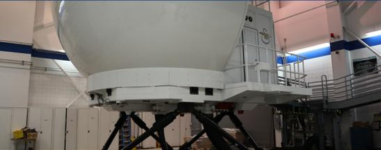
The Full Mission Simulator is a cutting-edge, aircraft-representative training solution that replicates the exact conditions of flying a BLACK HAWK aircraft. This advanced simulator combines authentic aircraft equipment with a six degree of freedom motion system and collimated display system.
