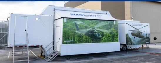
The Portable Flight Training Device is a compact, self-contained simulator that offers a cost-effective alternative to traditional full-flight simulators without requiring a facility. It can be ready within 8 hours of site arrival.
