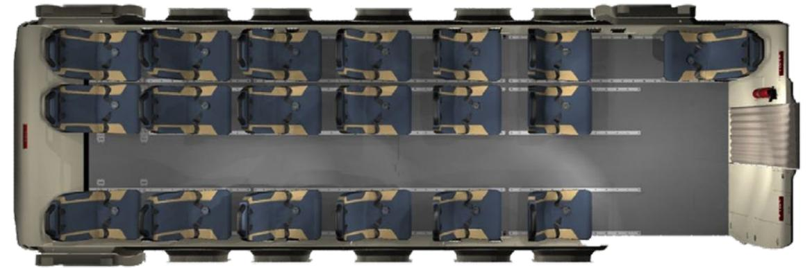
Sixteen (16) Passengers with Single Internal Auxiliary Fuel Tank
