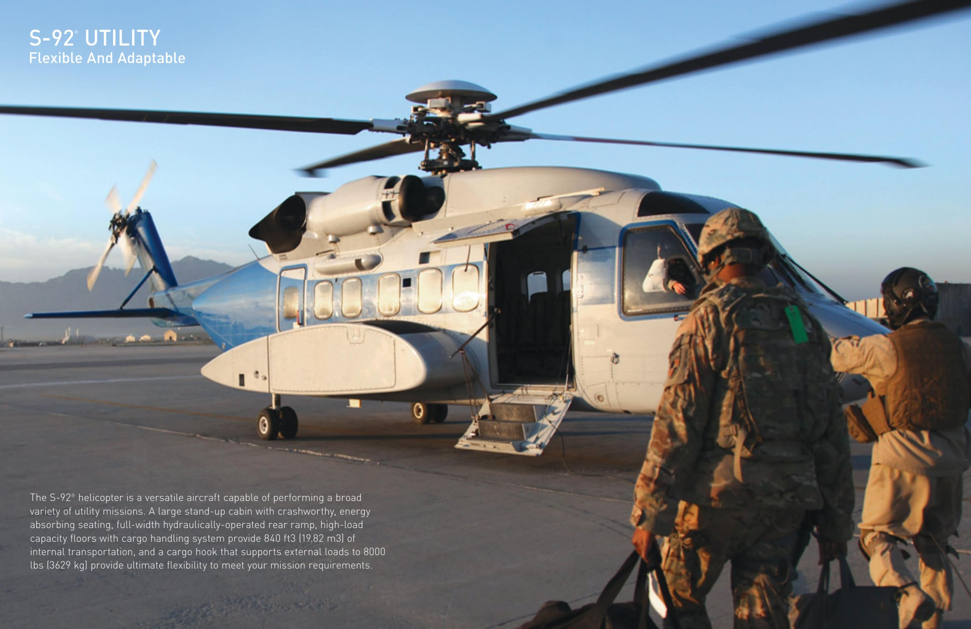
The S-92<sup>®</sup> helicopter is a versatile aircraft capable of performing a broad variety of utility missions. A large stand-up cabin with crashworthy, energy absorbing seating, full-width hydraulically-operated rear ramp, high-load capacity floors with cargo handling system provide 840 ft<sup>3</sup> (19.82 m<sup>3</sup>) of internal transportation, and a cargo hook that supports external loads to 8000 lbs (3629 kg) provide ultimate flexibility to meet your mission requirements.
